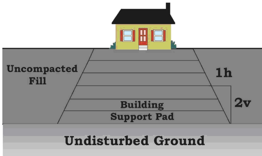
Figure 2. A representation of a "mine spoil pad" constructed to support an intended building site during reclamation. The spoil pad should extend beyond the minimum area required to support the actual building. In most cases, the zone where the surface is compacted should extend at least 10 feet beyond the intended footing area. The compacted spoil pad should extend downward at a minimum angle of about 30 degrees from the vertical (a 2v:1h slope).
