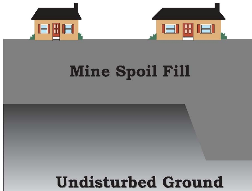
Figure 1. Settlement of underlying mine spoils can affect buildings constructed on mine spoil fills. The spoil depth under Building A is relatively uniform, whereas Building B is built over an area where spoil depth varies. Building B is more likely to be damaged due to differential settlement because it covers a larger lateral area, and because of variations in the depth of the underlying spoils.
